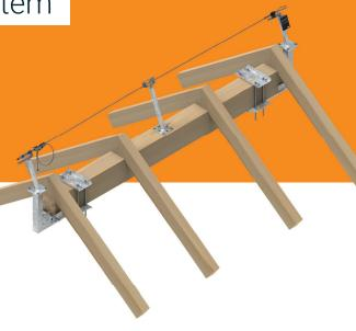
The temporary ridge safety system from INNOTECH is the perfect protective measure when setting up roof trusses. On the ground, the system is already attached to the wooden construction of the roof truss, and it provides protection to the installer on the ridge while he performs his work. In combination with personal protective equipment against falls from a height, the TFS system from INNOTECH is one of the
